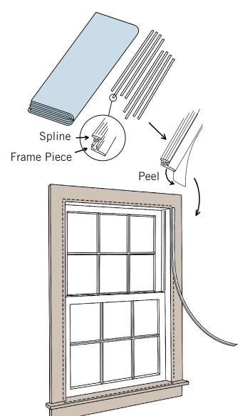
Peel the paper backing off each frame piece to expose the adhesive. Place along the penciled line and press firmly into place. Make sure it is placed exactly as you want, because the adhesive is strong and hard to move.
