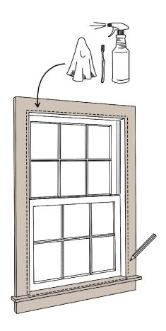
Remove any obstructions (blinds, latches, handles) that will get in the way of the plastic sheet once it's pulled tight.
