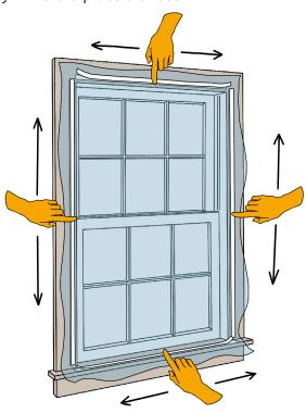
G Use scissors to cut off some extra plastic from the edges. If you plan to remove the plastic sheet each summer, don't cut too close to the edge to make reinstallation easier. You may want to label the plastic sheet in an unobtrusive corner so you know which window it belongs in when reinstalling.
