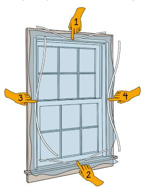
Cut out a piece of clear plastic that is at least four inches taller and wider than the frame. Zip a half inch of the plastic into the very center of the top edge of the frame. Zip a half inch into the center of the bottom of the frame, pulling the plastic tight. Zip a half inch into the center left side, then the center right side, pulling the plastic tight so there is no slack.
