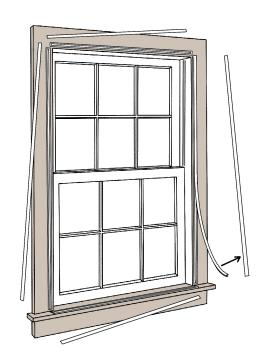
When you have the whole frame in place, unzip the spline from all the frame pieces.
